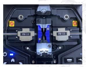
**2-12 cores metal fiber holder optional** Suitable for different type ribbon fibers
